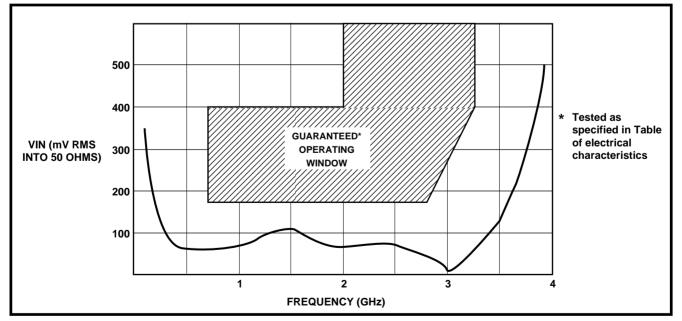
Figure 3 Typical input sensitivity
