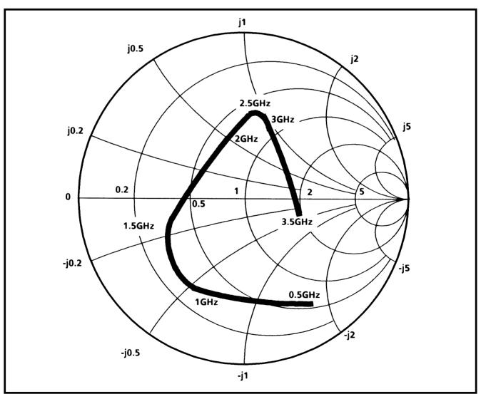
Figure 5 Typical input impedance
