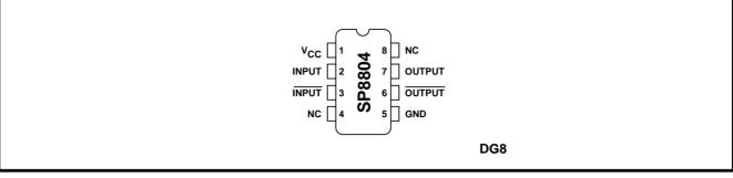
Figure 2 Pin connections
