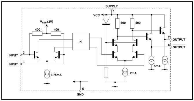
Figure 1 SP8804 Block diagram
