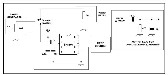
Figure 4 Test circuit
