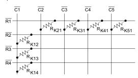
All the resistors are  $330k\Omega$ . The resistor option functions and the default specifications without option resistors are listed below.
